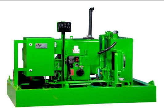
Engine : Electrically started Hatz silent pack diesel engine, type
