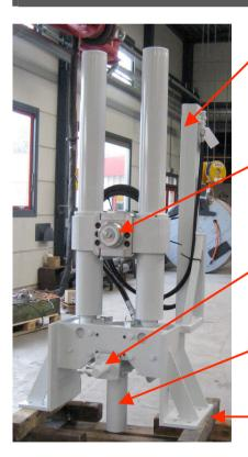
Guiding beam for hydraulic hoses, only supplied in combination with the hydraulic clamp
