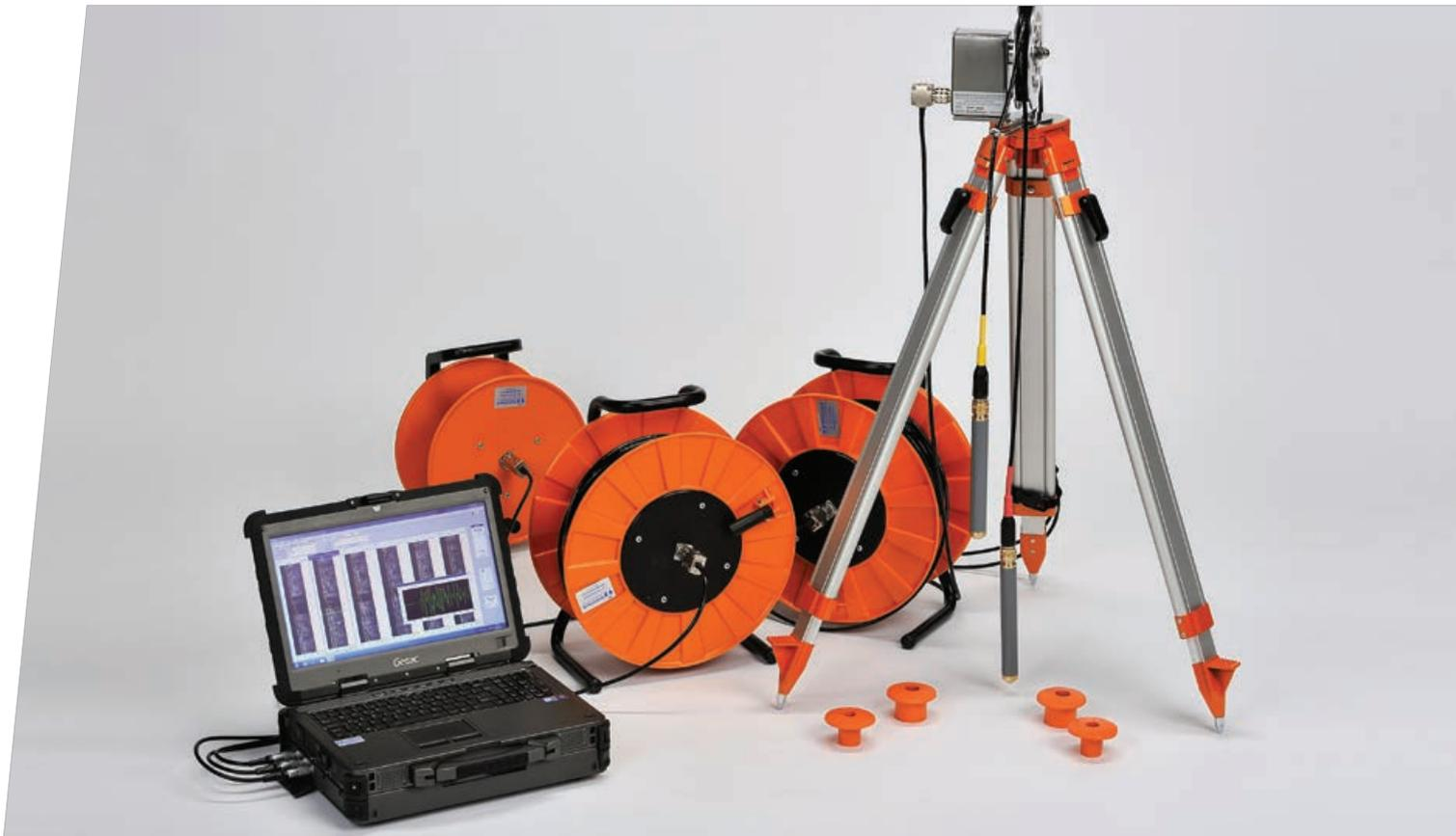
**SCXT3000 is a self-contained sonic logging system, suitable for testing concrete piles, barrettes and other mass concrete structures.**
